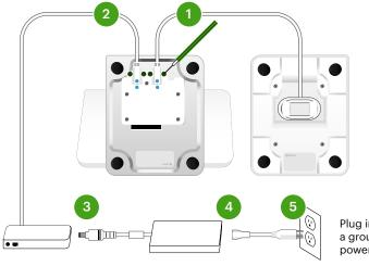
Plug in last, to a grounded AC power outlet.
